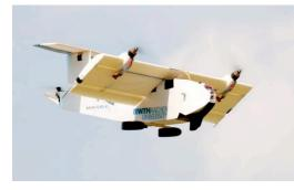
In a first approach, models with the Institute for Flight Dynamics at RWTH Aachen University have been developed and the software for the tilt-wing MAV has been implemented. With simple control concepts, the tilt-wing aerial vehicle could be stabilized in certain situations and a flight guidance system could be implemented. The onboard sensors of the prototype include an inertial measurement unit, a magnetometer, a GPS receiver, a barometer
