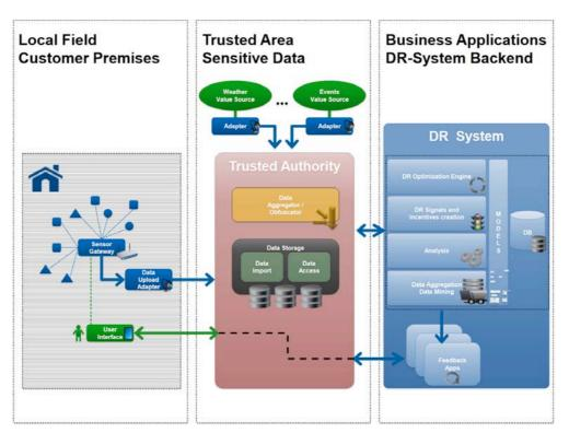
Fig. 3 - Conceptual Software Architecture
