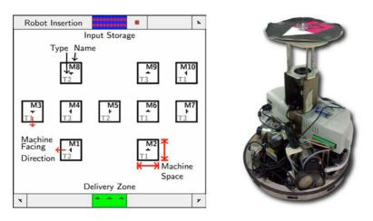
Figure 2: The left figure depicts the LLSF playing field, the right the modified Robotino robot of the Carologistics RoboCup team.
