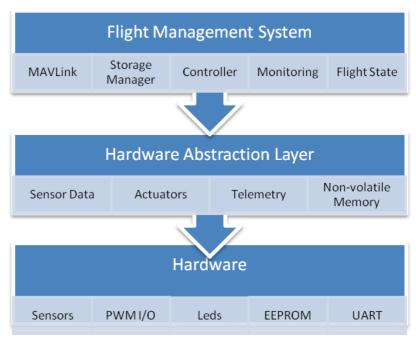
calculated and feed into the simulation, allowing software in the loop simulation. In the given figure, the hardware abstraction layer decides if the corresponding hardware shall be activated, or if data shall be sent to the simulator. Within the flight management system, there are systems taking care of storing control parameters (storage manager), the actual controller, monitoring techniques and the MAVLink protocol, to communicate to a ground control station.
