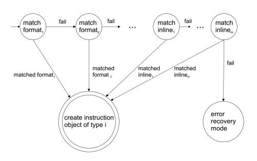
Figure 7.2: Mode of operation of the disassembler
