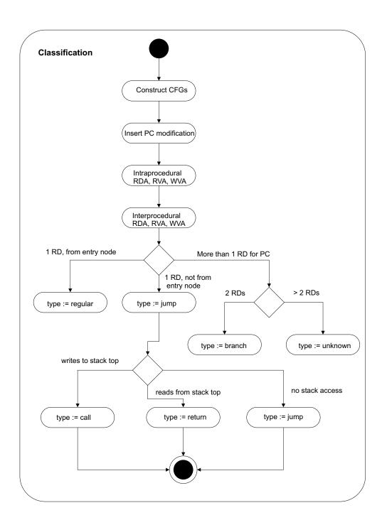
Figure 6.5: Instruction classification algorithm as an UML activity diagram. The outgoing edges from the final nodes for types *regular*, *branch* and *unknown* to the exit node have been omitted for clarity.
