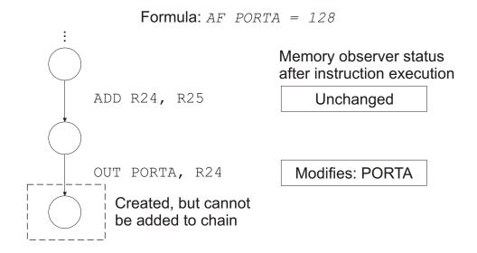
Figure 8.2: Monitoring of memory accesses in OTF Path Reduction
