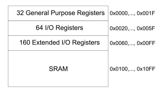
Figure 9.2: Memory layout of the Atmel ATmega644, as described and also illustrated in the device datasheet [7]
