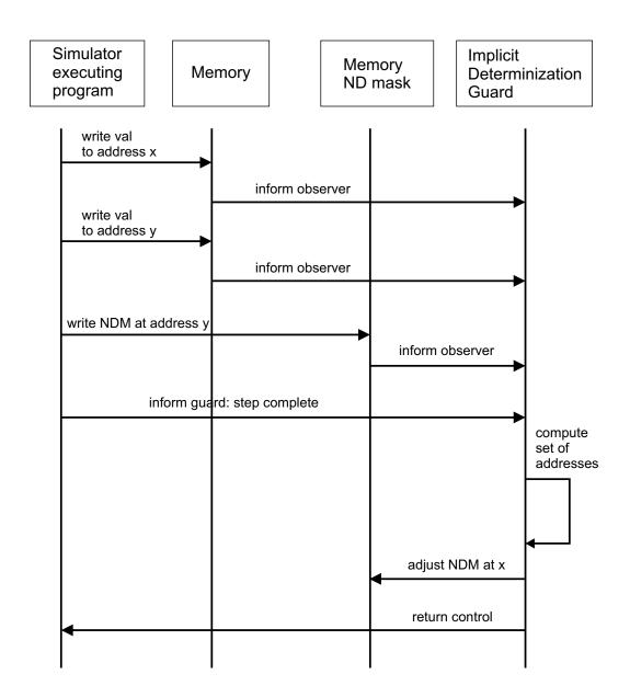
Figure 8.6: Message Sequence Chart illustrating the mode of operation of the Implicit Determinization Guard. During the step, the NDM of x is not explicitly modified, but the one for y is. Hence, the guard only performs a cleanup for x.
