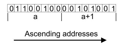
Figure 5.1: Interpretation of memory contents. The contents of the 8 bit cells a and a + 1 can be read as either two separate 8 bit values or a single 16 bit value. Furthermore, the ordering of the bytes may be swapped, with either a or a + 1 as the lowest byte in a 16 bit value. Other interpretations are also possible.
