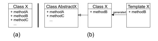
Figure 6.7: Replacement pattern for platform-dependent class X. (a) shows the starting point, with methodB being platform-dependent. (b) shows the situation after extracting the platform-independent code of X into AbstractX. The class X is now a generated class, created from a template file.
