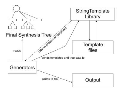
Figure 6.6: Structure of the backend for code generation in the SGDL compiler
