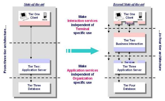
Figure 1. HIC Functional Architecture
