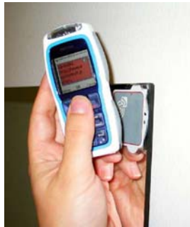
Fig 3. Touching the tag and initiating a context switch. In this case, the tag has been attached on a mirror next to the home front door.
