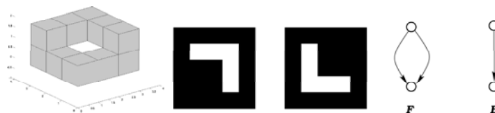
Fig. 2. A 5 \times 5 \times 4 binary volume with a torus, the corresponding slices and its connectivity graphs for foreground and background.
