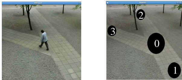
Figure 4. This figure firstly shows a frame of the video with a person taking a decision at the junction point, and secondly it shows where the virtual detectors are on the video.
