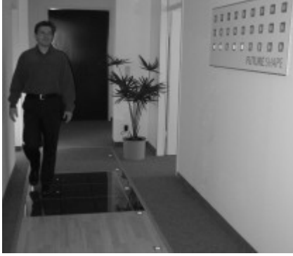
Fig. 3. Demonstrator with different floor coverings (carpet, glass, laminate). Walking on the floor wirelessly controls LEDs on the wall.
