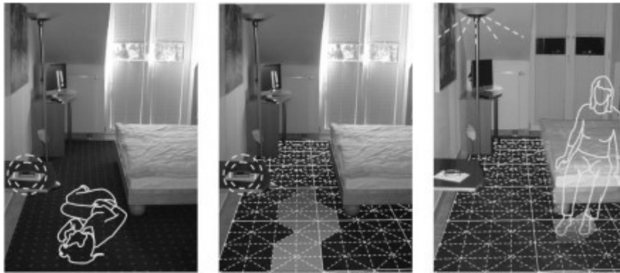
Fig. 5. By analyzing the movement trajectories and static sensor patterns, the floor can detect a fall. The room light is controlled based on peoples' behavior
