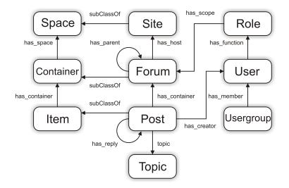
Fig. 1. Main classes and properties in the SIOC Core ontology.
