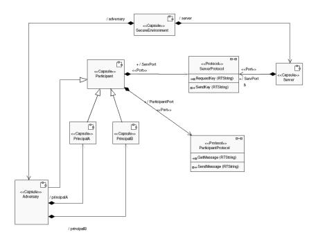
Fig. 1. Class Diagram of Participants in a Security Protocol
