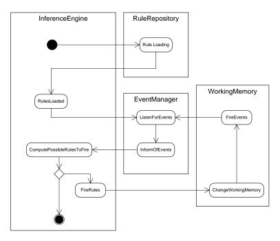
Fig. 5. The Rule Engine State Diagram
