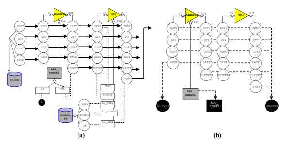
Fig. 2.3 Relationships of the architecture graph: (a) Part-of, provider and regulator relationships; (b) Instance-of relationships
