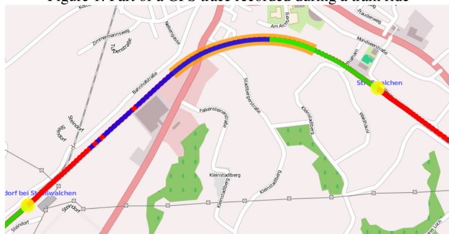
Figure 2: Automatically detected motion patterns in the GPS trace. (1) Standstill (yellow), (2) positive acceleration (green), (3) negative acceleration (red), (4) steady motion (blue), (5) negative course change (orange)
