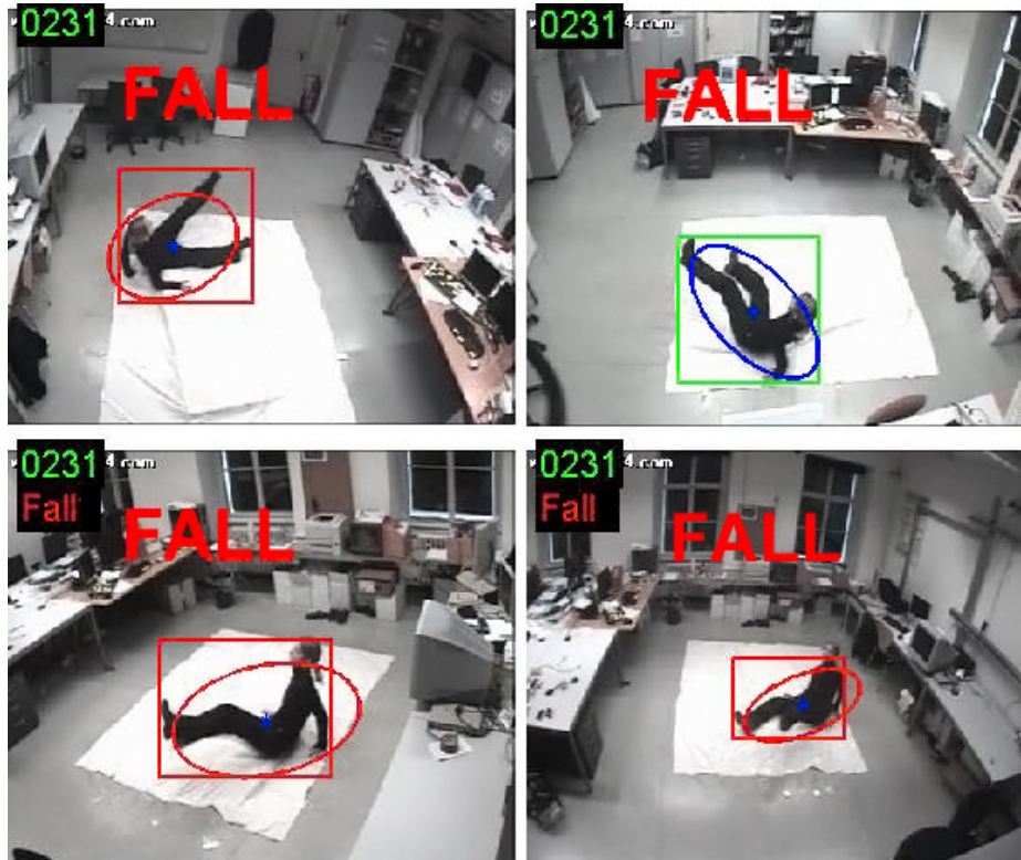
Figure 1. The four camera views of the test sequences with a person, showing the bounding box and fitted ellipse.
