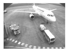
**Figure 6.** Snapshots of the ERA (Entrance Restricted Area) after completing Arrival-Preparation. The GPU (Ground Power Unit) and shocks are in place. The tanker crossing the ERA in the background (left) causes an erroneous interpretation thread (see text).
