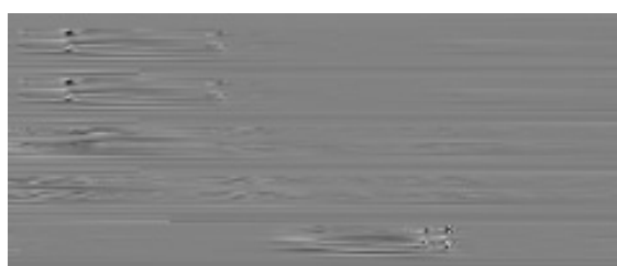
Figure 2. Excerpt from the raw data visualized as a greyscale bitmap. This figure shows 2 seconds of the example data set (horizontal) along 100 dimensions (vertical).
