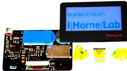
Figure 5. Name badge with IEEE802.15.4 radio transceiver, ultrasound transmitter and cholesteric LCD.
