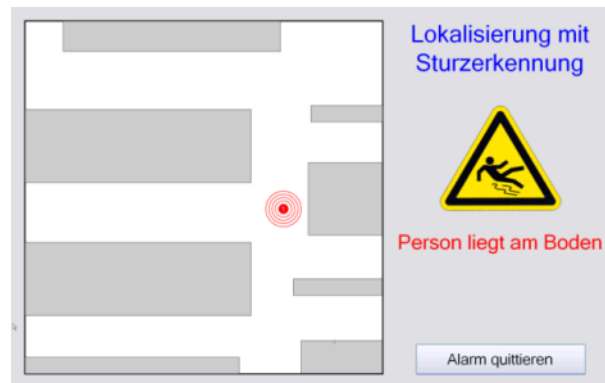
Figure 7. Fall detection application: The name badges transmit acceleration sensor data to the system. In case of a fall, an alert is generated, indicating the location of the incident.
