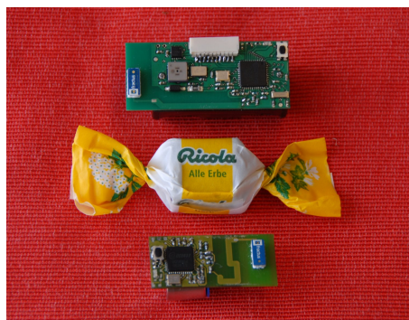
Figure 6. Small tags without display. Top: A device equipped with accelerometer and air pressure sensor [1]. Bottom: Simple transmitting device without sensors on board. Both tags are designed for long term operation.
