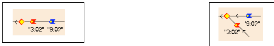
Figure 1. Two of the scenarios in which two trains could be arriving too close together at one infrastructural railtrack point
