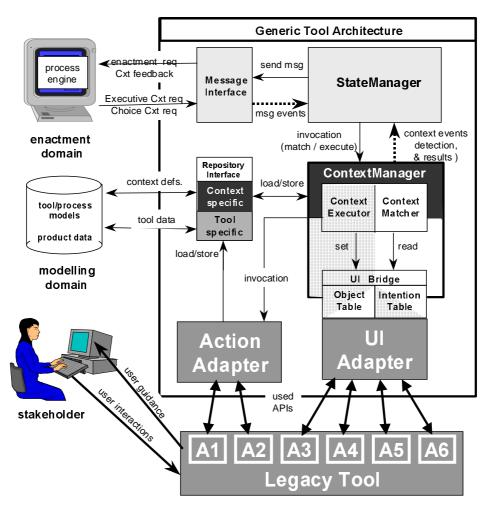
Figure 13: Adding adapter layers to the generic tool architecture for integrating legacy tools.
