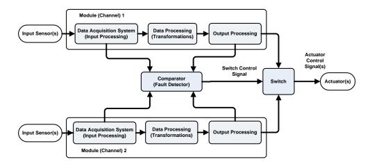
Figure 7.1.: Homogeneous Duplex Pattern
