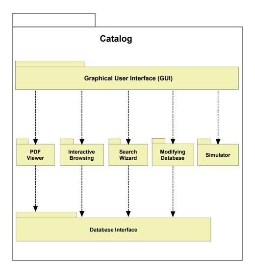
Figure 6.1.: The architecture of the catalog software.
