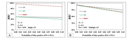
Figure 5.7.: The effect of the probability of false postive cases in AT on RRI.
