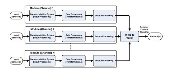
Figure 7.6.: M-out-of-N Redundancy Pattern
