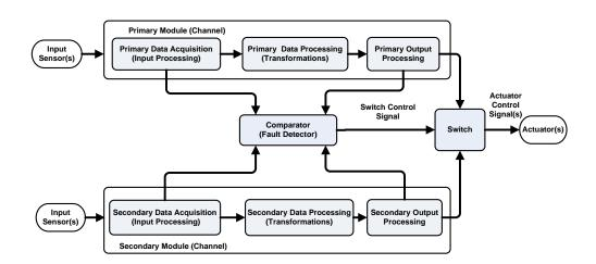
Figure 7.3.: Heterogeneous Duplex Pattern
