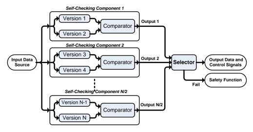
Figure 8.4.: N-Self Checking Programming Pattern
