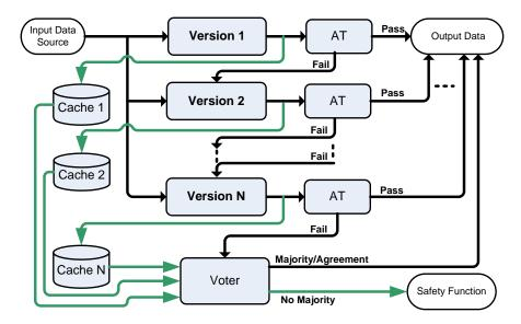
Figure 5.2.: Recovery block with backup voting method.
